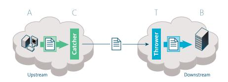
The diagram shows that system B (downstream) will never directly speak to system A (upstream) – communications go via the catcher and thrower. This means that an attacker must undergo a long chain of attacks to reach system B. At first glance, you might conclude that the catcher and the thrower only make the attack on system B somewhat more cumbersome but not impossible. **There is an ingenious way of preventing this.**
