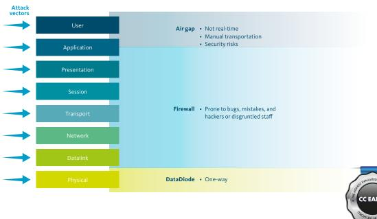
The network boundary options: Firewall > Air gap > DataDiode
